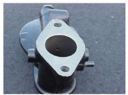
The small hole in the throat of the upper casting allows air to flow into the idle circuit when the throttle is closed. The throttle plate closes such that half of the hole just peeks above the closed throttle plate.
